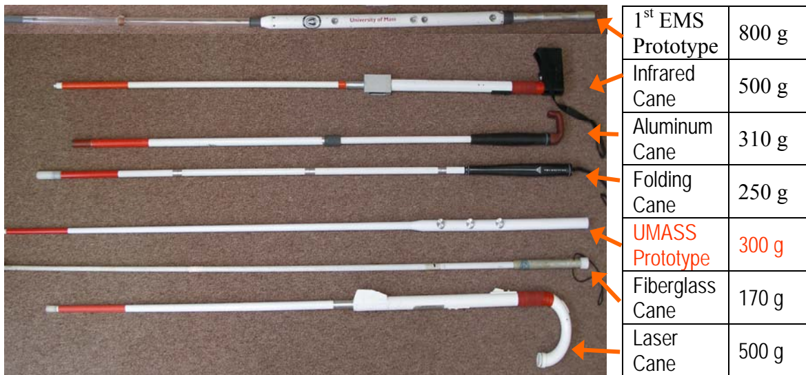
Figure 25: The new cane side-by-side with standard long canes and the earlier EMS cane.
