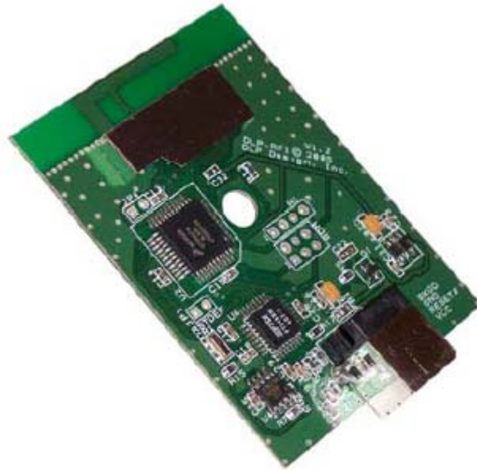
Figure 32: The DLP Design DLP-RF1-Z USB port transceiver
